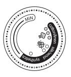
**NOTE:** The Temperature Dial does not adjust the amount of steam. Also, steam will only work at the specified temperature settings when set to ● ● or 🥋
