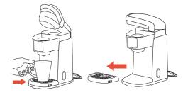
5 Close by pressing down on top of the Handle, making sure it is completely closed. The capsule will be punctured on top and the bottom when closing the Brew Head.
