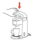
6 Press the "On/Off" button to start brewing coffee. During brewing, the "On/Off" button light will flash. The brewing process will take about 3 minutes.
