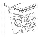
**3** Press Adapter (A/B/C) onto the vacuum bag valve. Connect one end of a Vacuum Tube to the appliance, the other to the Adapter.
